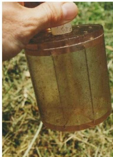
**Flowcell in use and exposed slides in insert**
