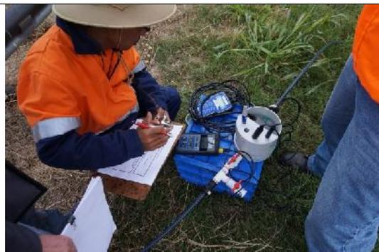
**CSGCU flow cell unit in use**
