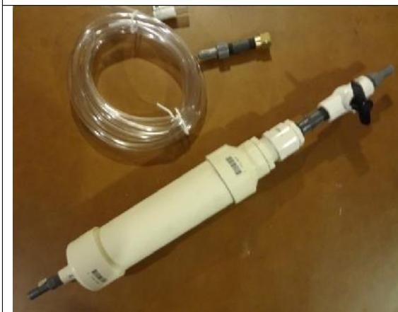
**Flowcell made from common plumbing parts**
