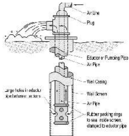
**Figure 2. Cable tool systems with double surge block airlift tools. A. Above-ground systems and a view of the tool. B. A diagram of the tool in action.**
